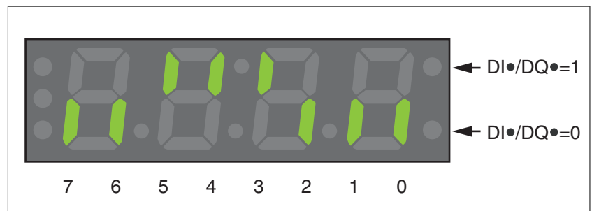
Figure 40: Integrated HMI, displaying the signal state of the digital inputs (DI•) and outputs (DQ•)
