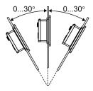
When installing this product in a slanted position with an incline more than 30°, the ambient temperature must not exceed 40 °C (104 °F). You may need to use forced air cooling (fan, A/C) to ensure the ambient operating temperature is 40 °C or less (104 °F or less).
